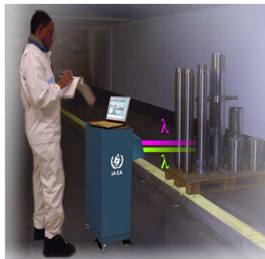
FIG. 7. A trained IAEA inspector operates the LIBS unit on-site. The spectroscopic profile is compared to those in its library to determine material's make-up and history.
