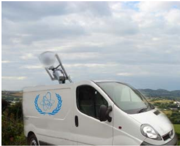
FIG. 10. A mobile on-site laboratory samples and concentrates atmospheric-borne pollutants. Local meteorological conditions and the GPS location are also recorded.
